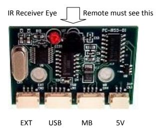
From the back of the IRS5, starting on the right, the connectors are:
